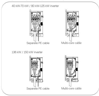
b. Re-install the cover of wiring box and tighten it with screws (with the torque of 5-7 N·m).
