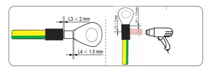
> Step 2: Connect the grounding cable to the inverter.
