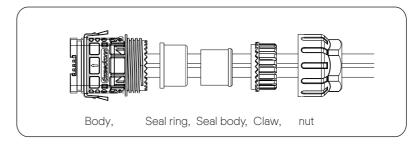
e. Insert the tube type terminal into the housing according to the label on it. Push the terminal-inserted housing into the body. There will be a slight sound of "Click", which indicates the connection is completed.
