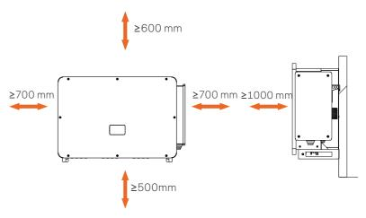
For multi-inverter installation, please reserve the space of 1200 mm at least between each left and right inverter and at least 500 mm between each upper and lower inverter.
